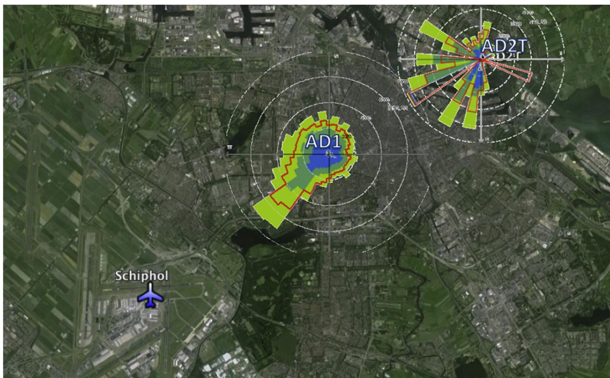
**Fig. 10.** Locations of the fixed (AD1) and mobile unit (AD2M) monitoring sites at respectively 8 and 14 km from Schiphol airport, with pollution roses of the wind direction averaged (red) 10–20 nm concentration per site. (For interpretation of the references to colour in this figure legend, the reader is referred to the web version of this article.)
